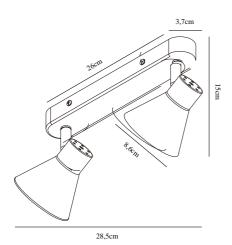
Voltage (V): 230 Volt IP degree if the fixture includes two types of IP degree: IP20 Maximum compatible bulb wattage (W): 35W Class (Class I, Class II, Class III): Class 1 (Earth contact) Lampholder type (eg, E27/E14, etc): GU10 Dimmerable: Yes with compatible
