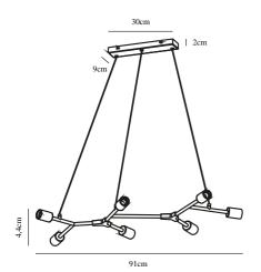
Voltage (V): 230 Volt IP degree if the fixture includes two types of IP degree: IP20 Maximum compatible bulb wattage (W): 60W Class (Class I, Class II, Class III): Class 2 (Double isolated) Lampholder type (eg, E27/E14, etc): E27
