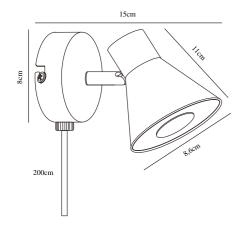
Voltage (V): 230 Volt IP degree if the fixture includes two types of IP degree: IP20 Maximum compatible bulb wattage (W): 35W Class (Class I, Class II, Class III): Class 2 (Double isolated) Lampholder type (eg, E27/E14, etc): GU10
