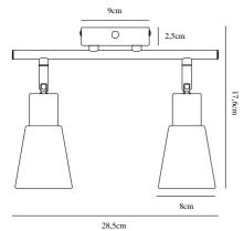
Voltage (V): 230 Volt IP degree if the fixture includes two types of IP degree: IP20 Maximum compatible bulb wattage (W): 40W Class (Class I, Class II, Class III): Class 2 (Double isolated) Lampholder type (eg, E27/E14, etc): E14
