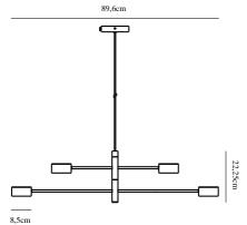
Voltage (V): 230 Volt IP degree if the fixture includes two types of IP degree: IP20 Class (Class I, Class II, Class III): Class 2 (Double isolated) Lampholder type (eg, E27/E14, etc): LED Module
