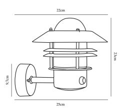
Voltage (V): 230 Volt IP degree if the fixture includes two types of IP degree: IP54 Maximum compatible bulb wattage (W): 60W Class (Class I, Class II, Class III): Class 1 (Earth contact) Lampholder type (eg, E27/E14, etc): E27 Parallel connection possible?: True
