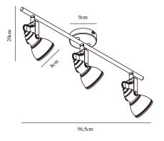
Voltage (V): 230 Volt IP degree if the fixture includes two types of IP degree: IP20 Maximum compatible bulb wattage (W): 35W Class (Class I, Class II, Class III): Class 2 (Double isolated) Lampholder type (eg, E27/E14, etc): GU10 Dimmerable: Yes with compatible bulb
