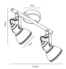
Voltage (V): 230 Volt IP degree if the fixture includes two types of IP degree: IP20 Maximum compatible bulb wattage (W): 35W Class (Class I, Class II, Class III): Class 2 (Double isolated) Lampholder type (eg, E27/E14, etc): GU10 Dimmerable: Yes with compatible
