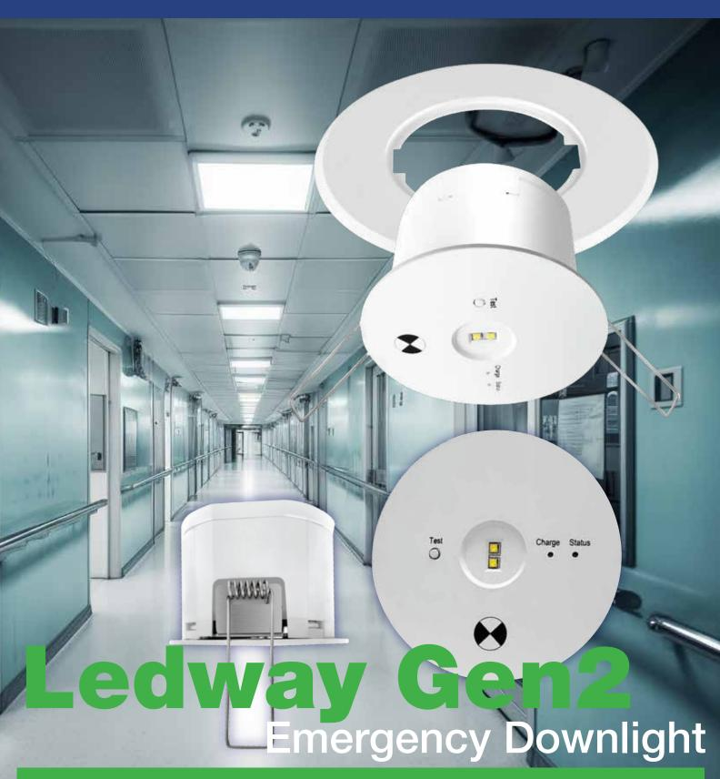
As an integrated Non-Maintained Emergency Downlight, Ledway Gen 2 has been designed with the installer in mind. Ledway Gen 2 will fit multiple ceiling cut-outs from 73-120mm and comes complete with a ceiling adaptor to retrofit into 145mm cut-outs. The Ledway Gen 2 has a D63 classification and 1200mm Flex & Plug
